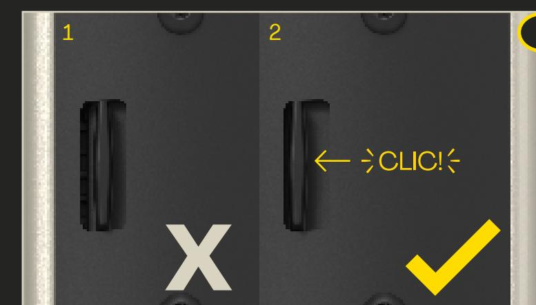
**i** LA PORTE DE RANGEMENT DOIT ÊTRE CORRECTEMENT ENCLANCHEE POUR GARANTIR SA FIXATION AU NIVEAU DE LA DIAGONALE.
