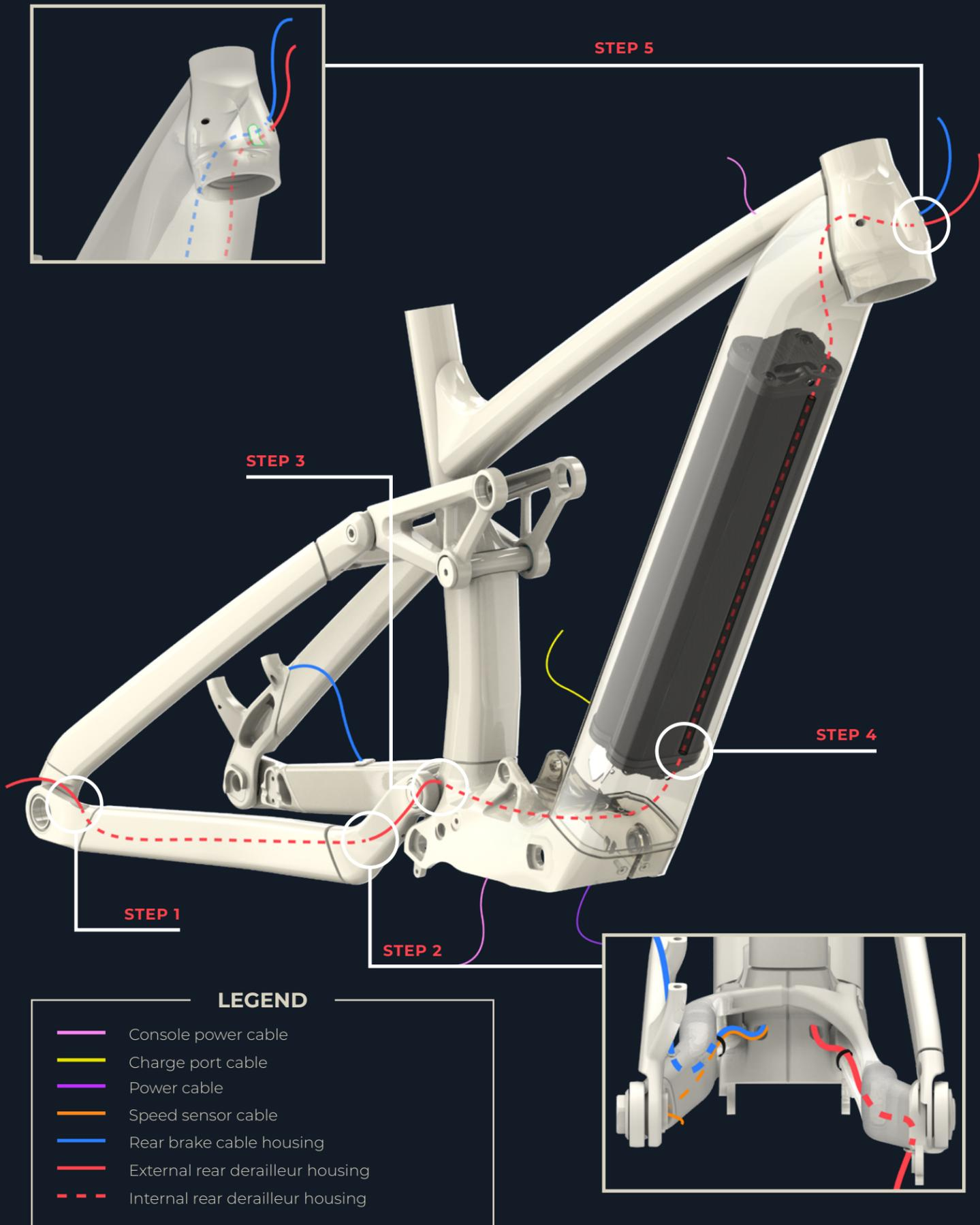
**i** Make sure the battery is in place in the down tube before starting.
