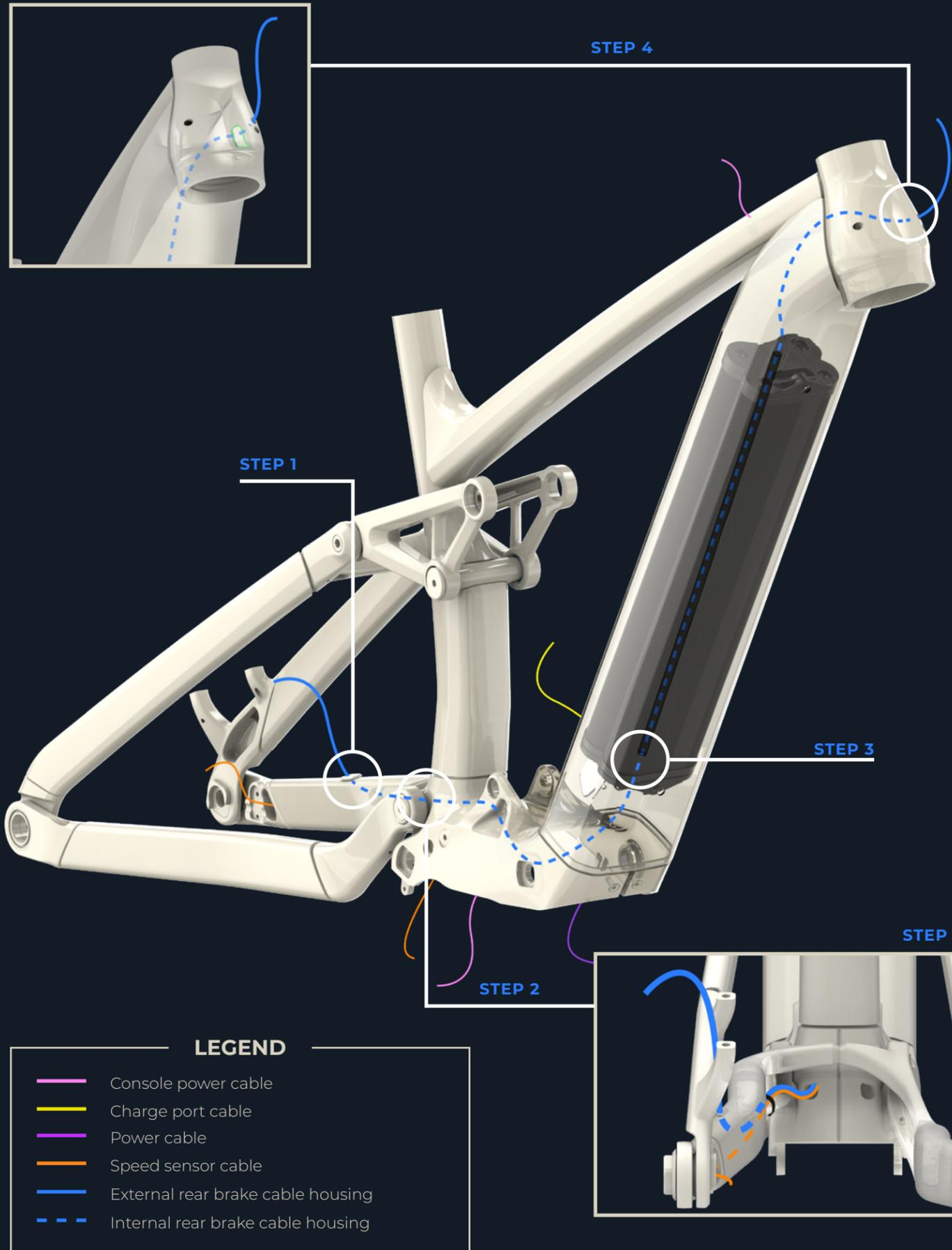
**i** Make sure the battery is properly installed in the down tube before starting.
