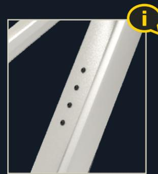
The **lower** position of the inserts is reserved for the **water bottle holder**, while the **upper** position is exclusive to the Bosch **powermore** battery extension.
