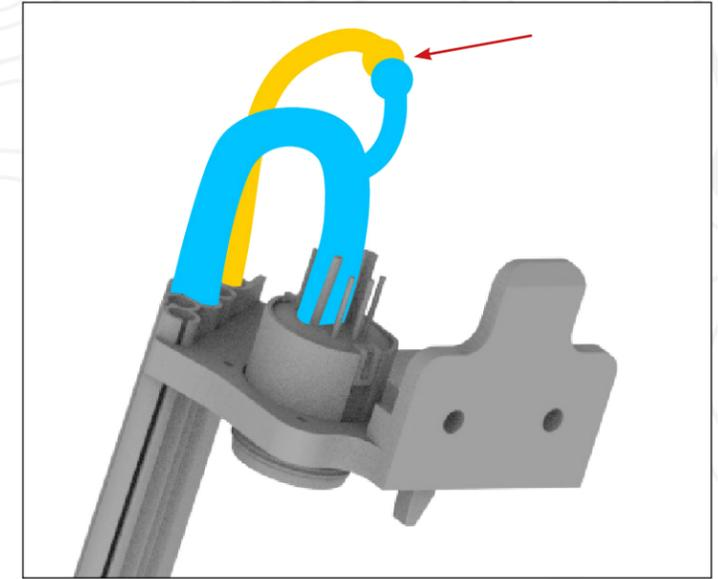
**Step 4.2 | Step 2.2 | Step 3.2 |** Introduce the cables into the cable guide while making sure to nest the wires in their respective base. (See annex 1.1)
