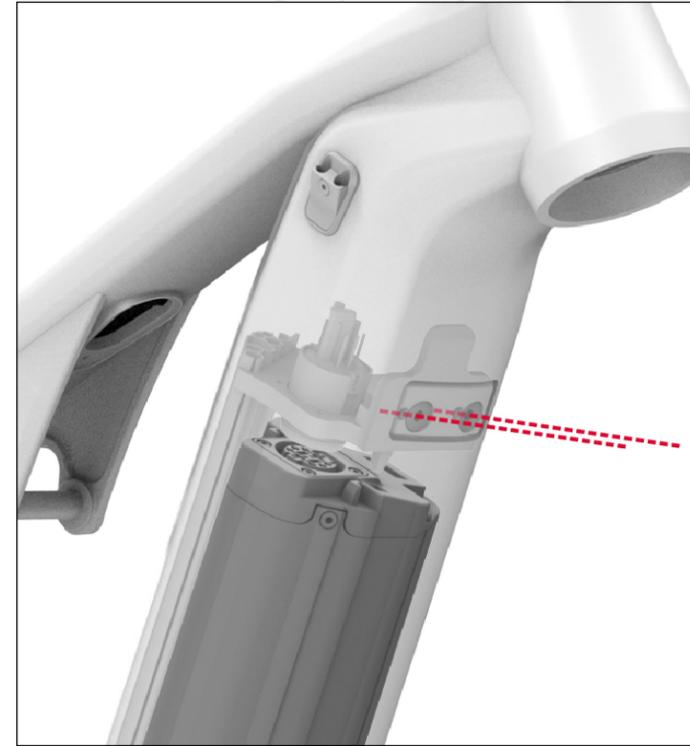
**Step 4.4 | Step 2.4 | Step 3.4** | Once the cable guide is fully inserted in the diagonal, ensure that it is correctly positioned by guiding you using the battery.
