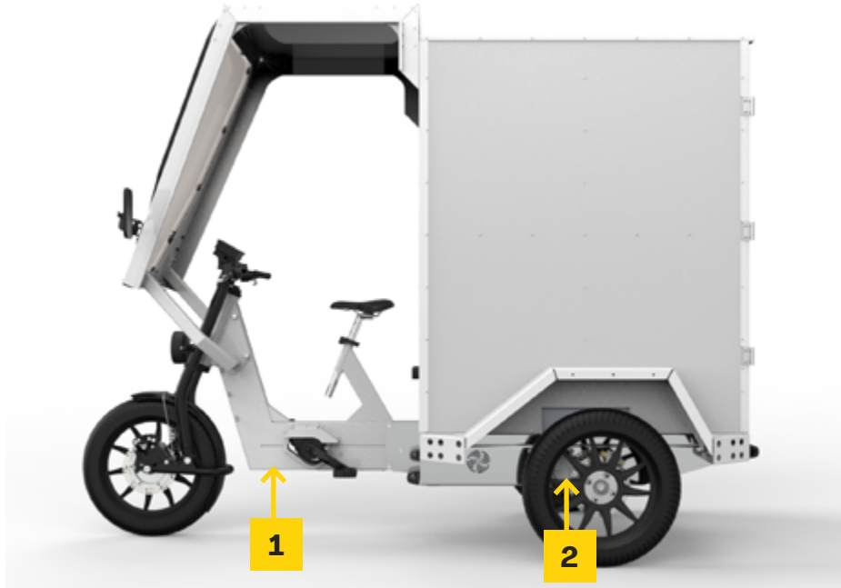
FIGURE 19 : JACK SUPPORT POINT
