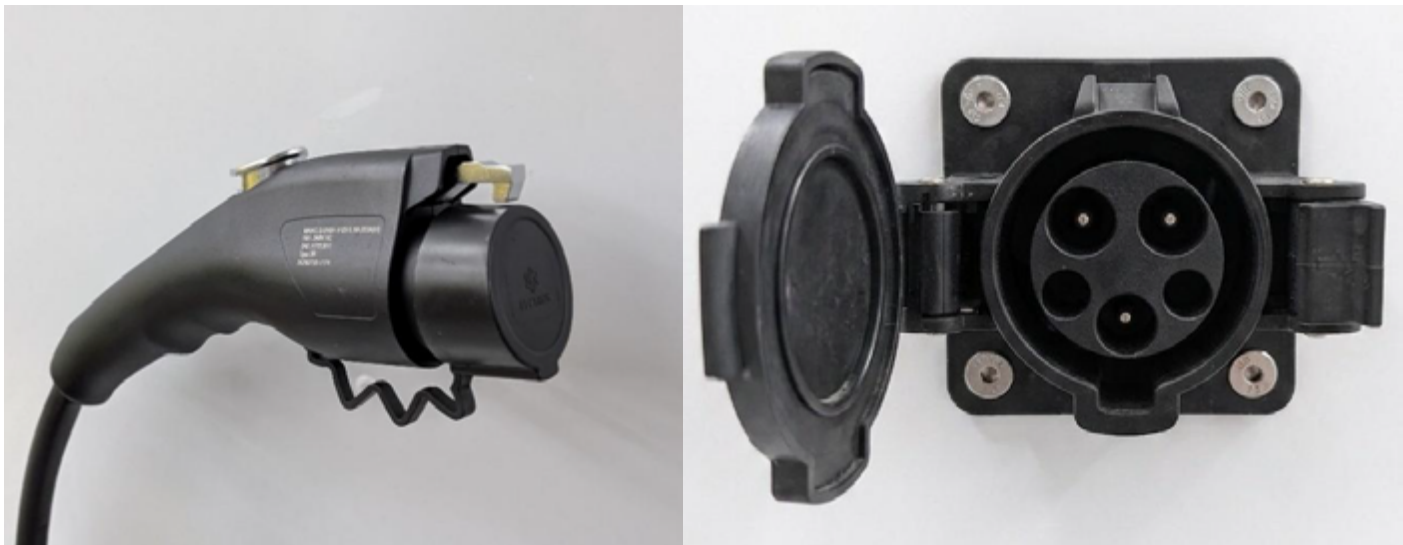
FIGURE 13 : FIL CHARGING CABLE AND CHARGING PORT
